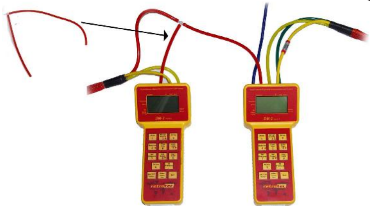
Blower Door gauge DucTester gauge
