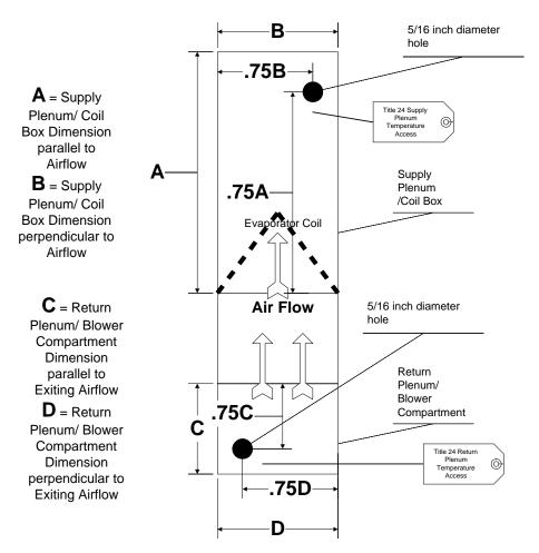
Each location shall have a 5/16" (8 mm) diameter hole. The supply location shall be labeled "Title 24 – Supply Temperature Access" in at least 12-point type. The return location shall be labeled "Title 24 – Return Temperature Access" in at least 12-point type. These locations can be in any one of the four sides of the plenums.
